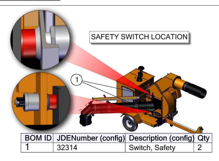
SAFETY SWITCHES NEED TO BE CHECKED FOR CORRECT OPERATION BEFORE EACH USE. DO NOT OPERATE MACHINERY WITH MALFUNCTIONING SAFETY SWITCHES. FAILURE TO COMPLY COULD RESULT IN SERIOUS PERSONAL INJURY OR DEATH.
